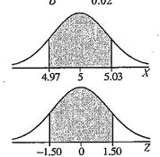
From Table V, the area to the left of  $z_1 = -1.50$  is 0.0668 and the area to the left of  $z_2 = 1.50$  is 0.9332, so  $P(4.97 \le X \le 5.03) = 0.9332 - 0.0668 = 0.8664$ . So, 0.8664, or 86.64%, of the ball bearings manufactured will be between 4.97 and 5.03 mm. Let n represent the number of ball bearings that must be manufactured. Then 0.8664n = 50,000,
