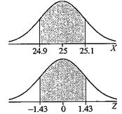
From Table V, the area to the left of  $z_1 = -1.43$  is 0.0764 and the area to the left of  $z_2 = 1.43$  is 0.9236, so  $P(24.9 \le X \le 25.1) = 0.9236 - 0.0764 = 0.8472$ . [Tech: 0.8469] So, 0.8472, or 84.72%, of the rods manufactured will be between 24.9 and 25.1 cm. Let n represent the number of rods that must be manufactured. Then, 0.8472n = 10,000,
