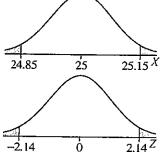
From Table V, the area to the left of  $z_1 = -2.14$  is 0.0162, so P(X < 24.85) = 0.0162. The area to the left of  $z_2 = 2.14$  is 0.9838, so P(X > 25.15) = 1 - 0.9838 = 0.0162. So, P(X < 24.85 or X > 25.15) = 2(0.0162) = 0.0324. [Tech: 0.0321] The proportion of rods that will be discarded is 0.0324, or 3.24%.
