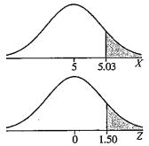
From Table V, the area to the left of z = 1.50 is 0.9332, so P(X > 5.03) = 1 - 0.9332 = 0.0668. So, the proportion of ball bearings that has a diameter more than 5.03 mm is 0.0668, or 6.68%.
