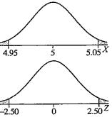
From Table V, the area to the left of  $z_1 = -2.50$  is 0.0062, so P(X < 4.95) = 0.0062. The area to the left of  $z_2 = 2.50$  is 0.9938, so P(X > 5.05) = 1 - 0.9938 = 0.0062. So, P(X < 4.95 or X > 5.05) = 2(0.0062) = 0.0124. The proportion of ball bearings that will be discarded is 0.0124, or 1.24%.
