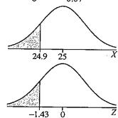
From Table V, the area to the left of z = -1.43 is 0.0764, so P(X < 24.9) = 0.0764. [Tech: 0.0766] So, the proportion of rods that has a length less than 24.9 cm is 0.0764, or 7.64%.
